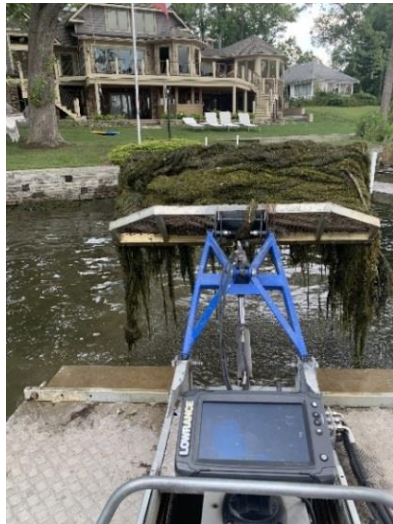
Photo of a Town of Chautauqua Mobitrac collecting plant debris (Source Mobitrac operator).
