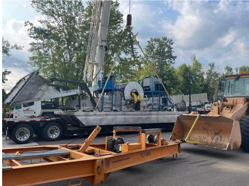
Figure 1. Pictured above, a crane places a new plant harvester purchased by Chautauqua County onto a trailer at the Chautauqua Lake Association shop in Lakewood. Photo by Jay Young.
