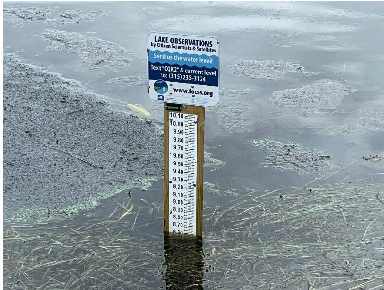
Figure 1. A new lake gauge from the Lake Observations by Citizen Scientists and Satellites program was added to the Prendergast Point boat launch on Chautauqua Lake on June 6, 2022.
