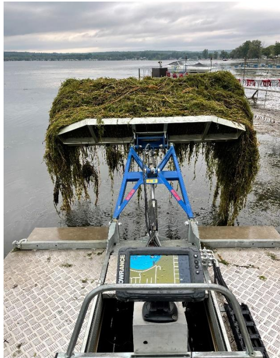
Figure 1. A Town of Chautauqua Mobitrac is pictured with a full rake of plants. An Alliance-monitored Lowrance sonar and GPS unit can be seen mounted center frame.
