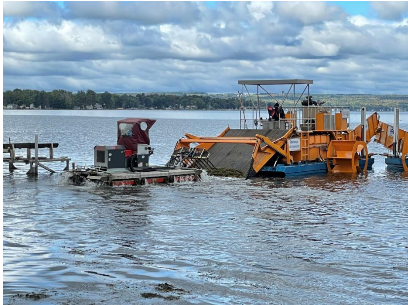
Figure 1. A Town of Chautauqua Mobotrac offloads to a Chautauqua Lake Association vessel during 2021 in-lake maintenance joint operations.
