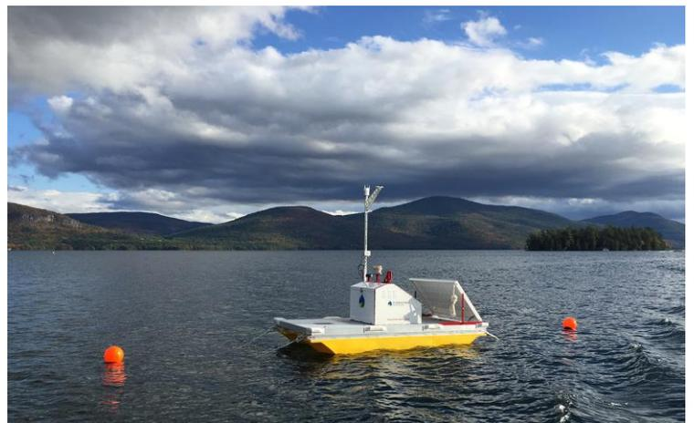
**Photo 2.** One of two Rensselaer Polytechnic Institute-built vertical profilers that will be installed on Chautauqua Lake in late-August (Source: Rick Relyea).
