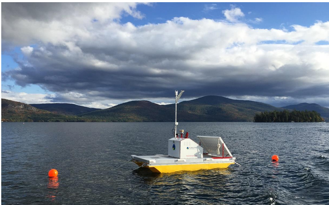
Photo 1. One of two Rensselaer Polytechnic Institute-built vertical profilers that will be installed on Chautauqua Lake in late-August (Source: Rick Relyea).
